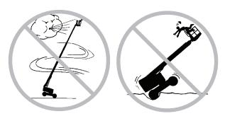
the machine in stowed position across uneven terrain, debris, unstable or slippery surfaces and near holes and drop-offs.
