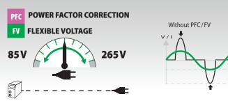
The TIG 200 DC has a powerful integrated PFC and features FLEXIBLE VOLTAGE (85-265V).
