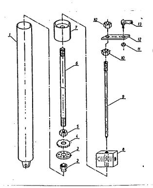
Should the saw frame still lower even at correctly adjusted rods, the reason must be dirt in the nozzle or sleeve (3) is worn out.
