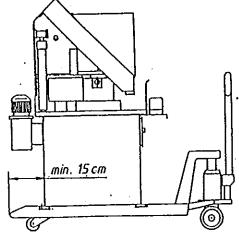
Before the transport the machine has to be cleaned from chips and loose metal parts.
